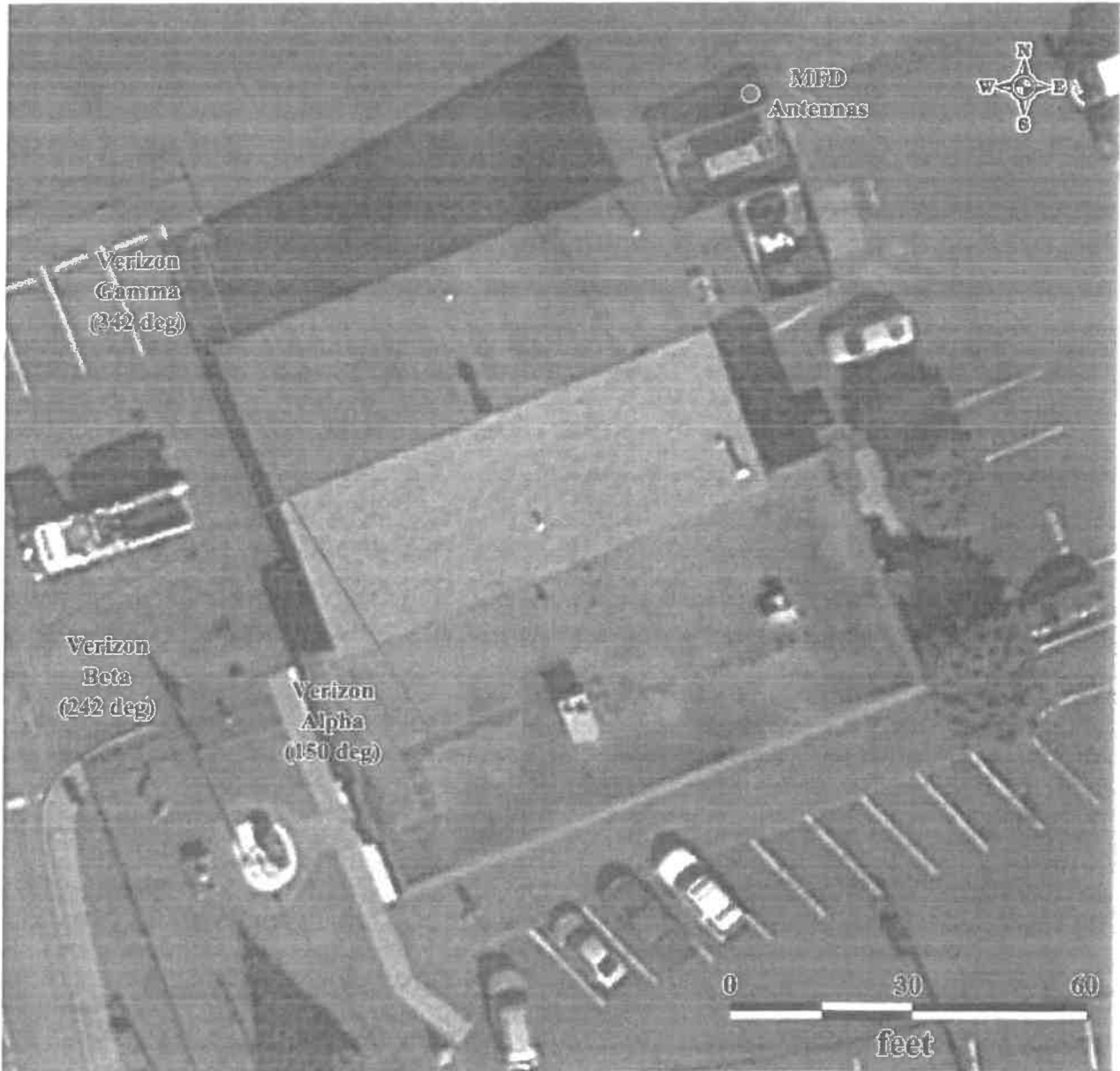
Figure 1: Verizon Antenna Location & Azimuths
