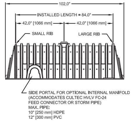
CULTEC RECHARGER 330XLHD CHAMBER STORAGE = 7.459 CF/FT [0.693 m³/m]
